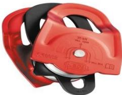
**Description:** Special side plates designed for use with a Prusik friction hitch in progress capture systems. Parallel mounted sheaves and auxiliary attachment point for creating different types of hauling systems, including the most complex. Accepts up to three carabiners to facilitate use. Certification(s): CE EN 12278, NFPA 1983 General Use
